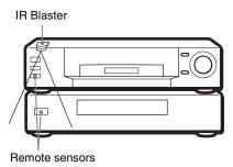
If the infrared receivers on the two video devices do not line up like the illustration above, you need to purchase an optional IR Blaster (VM-50, not supplied) and install it.
